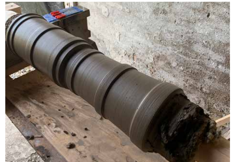
Fig. 4-6. 3 stages in producing the cannon mould
