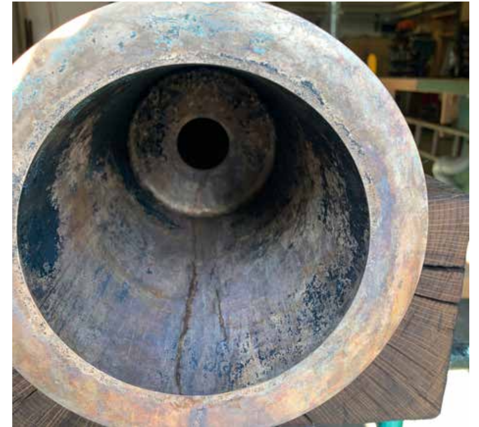
Fig. 17. Few signs of use in the barrel after the shootings.
