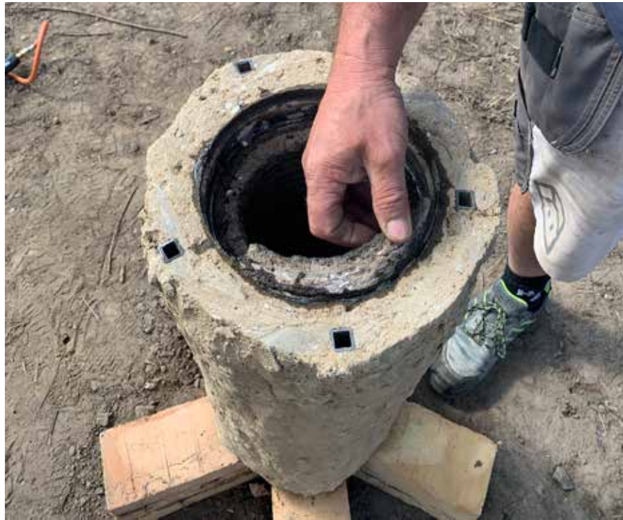
Fig. 7. Removing the inner form after baking the mould.
