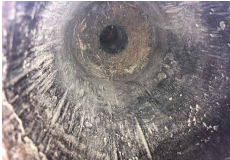
Fig. 2. Longitudinal striations in the cannon from use
